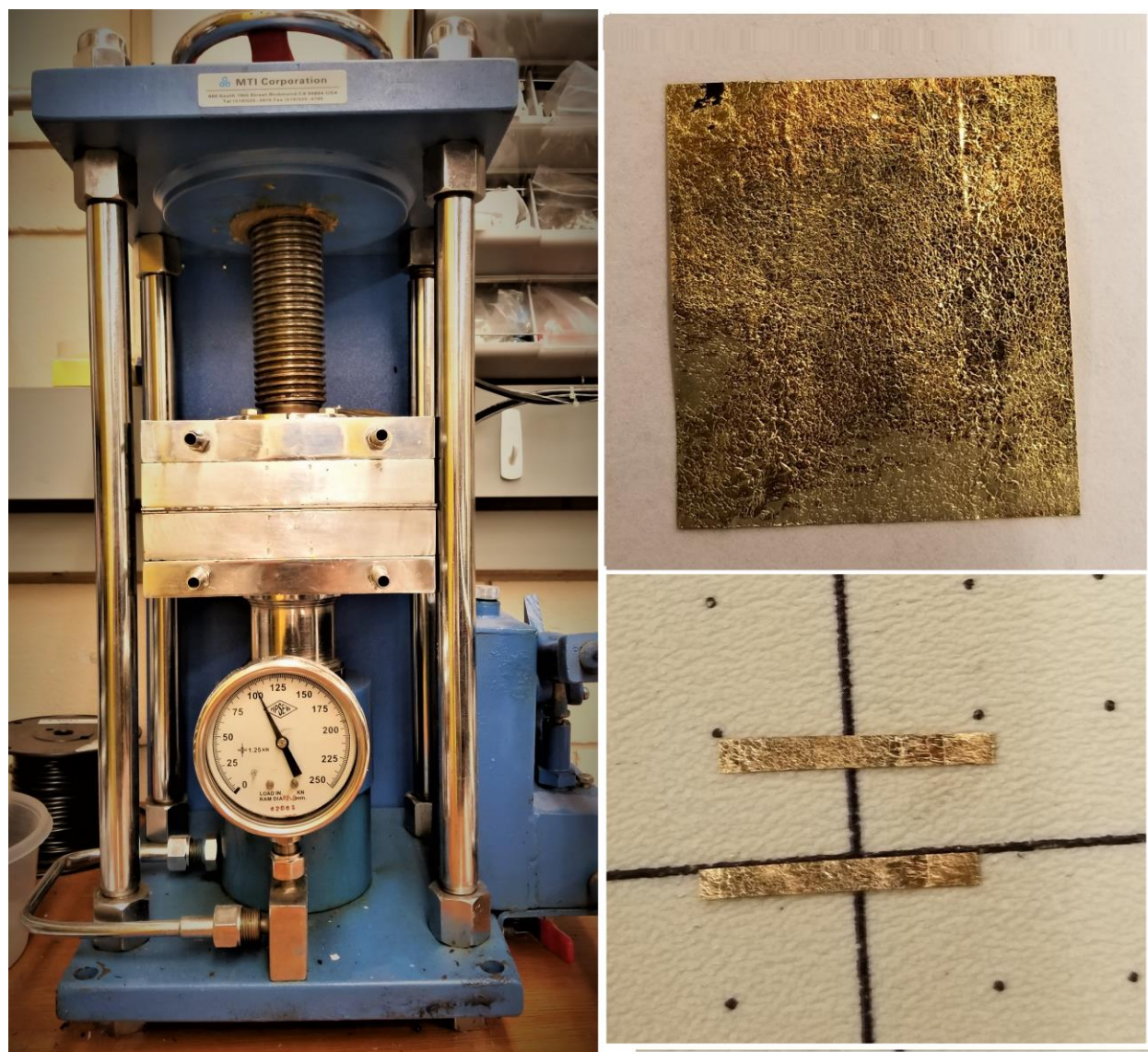
Figure 2-6: 25T hydraulic hot press machine (left), final hot pressed membrane (right, upper), and actuators to be tested (right, lower)
