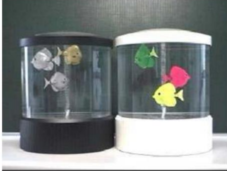
Figure 1-2 : First commercial EAP actuators in swimming fish. Produced in Japan in 2002 by Eamex.
