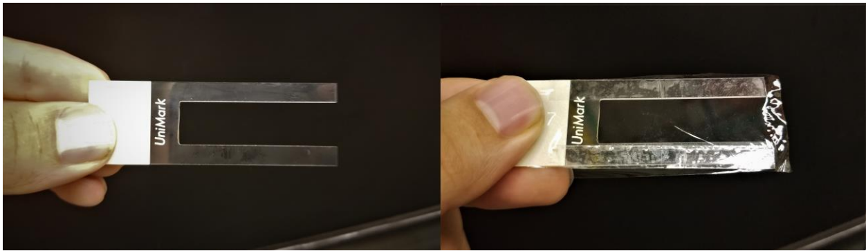
Figure 2-2: Glass frame used to hold the membrane during LbL ionic self-assembly process (left). Nafion membrane attached to a glass frame (right)
